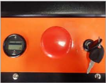
Timer & Emergency Stop Switch & Power Switch
