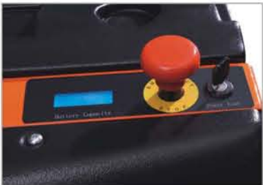
Timer & Emergency Stop switch & Power switch
