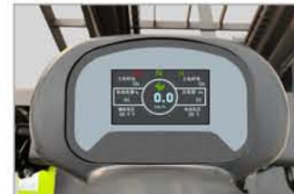
Multi function LED display, vehicle status is clear at a glance
